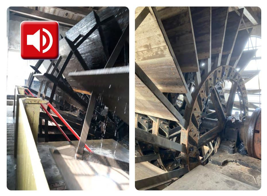
Three scoop wheels turn in each scoop wheel house. Together, they displace 1.5 million litres of water per minute. The maximum lifting height is 60 cm. A scoop wheel has a diameter of 7.5 metres and a width of 2 metres. They
