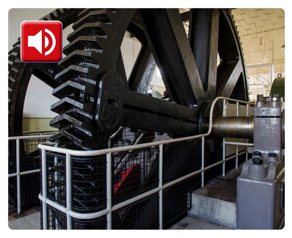
straight toothing, and there is less resistance and therefore less wear. The gearing still looks fine and has never been replaced. Herringbone gearing was invented by André Citroën while he was still working in a machine factory. When he opened a car factory, he put two herringbone teeth as a
