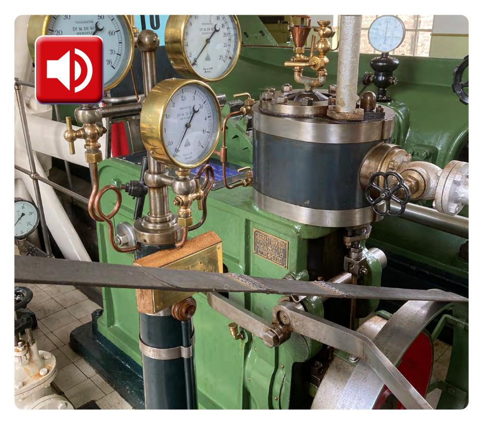
movement. The operator then quickly uses the large horizontal wheel to open the main shutoff valve to release the steam into the cylinder.
