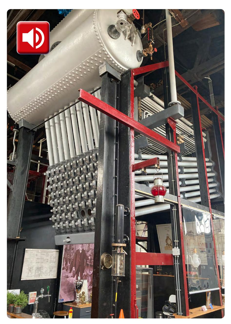
pipes, the steam left the boiler at a temperature of 330 degrees through a steam pipe on its way to the steam engine. More on that later. You can now move on from the dismantled boiler to the model table.
