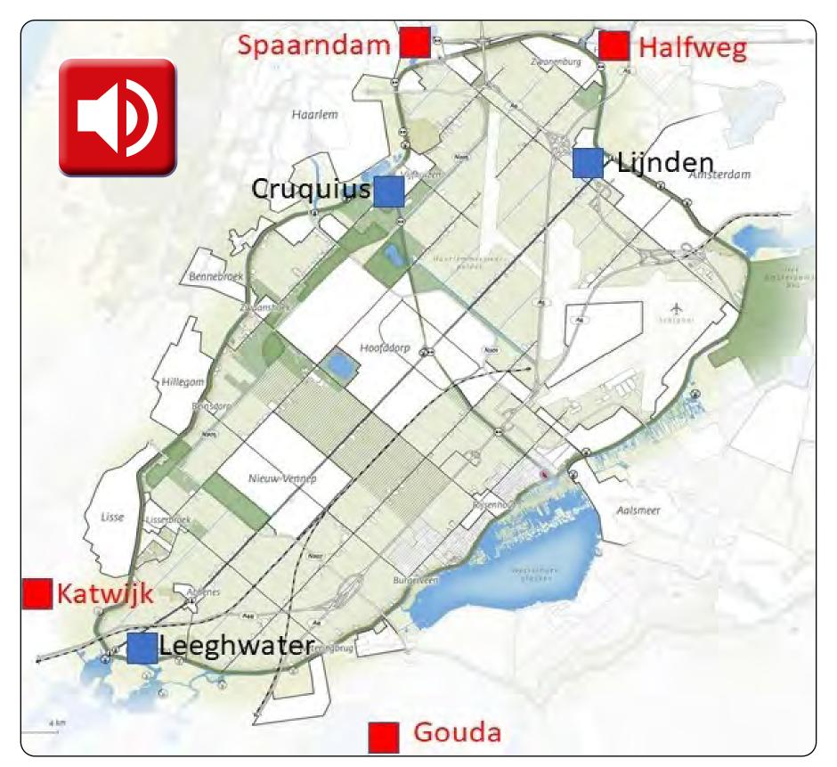
How did this reclamation work? First, a dyke was built around the inland sea, with a ring canal being dug behind this dyke. Everything was done by hand, with shovels and wheelbarrows, and took a total of eight years to complete. The result was a ring canal, 59 km in length. Three polder pumping stations (blue block) subsequently pumped the water from the polder into the ring canal, leading to the drying up of the lake in 1852. With four other
