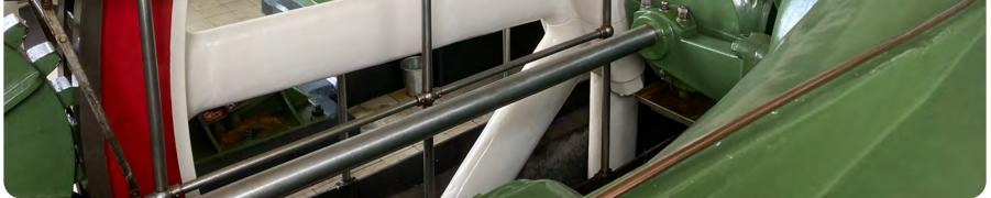
At both ends of the crankshaft, in the closed semi-circular green cabinets, gears are mounted to reduce the speed of rotation. This increases the force on the shaft of the scoop
